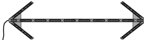
1. There is a slot along the length of the back of the arrowstick that should be used to facilitate mounting. Insert the heads of the two enclosed #10 carriage bolts into the hole in the slot.
